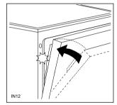
If the door does not close correctly, loosen or tighten the adjustable support feet, until the machine is perfectly level.
